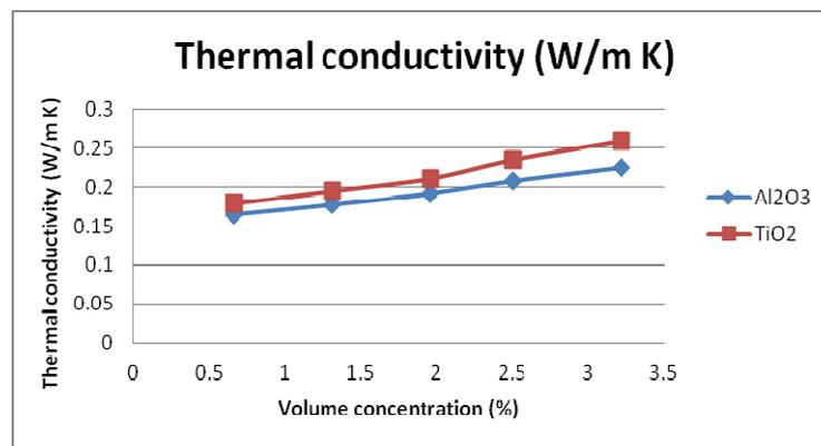
**Graph 1: Thermal Conductivity Graph where the Values on X-axis Denote the Volume Concentration of Nanoparticles and the Values on Y-Axis Denote Thermal Conductivities in Watt per Meter Kelvin.**
